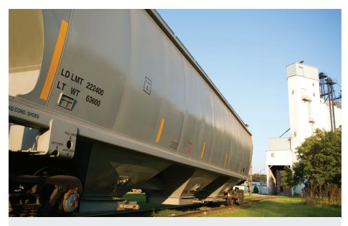
Covered hopper cars, which are fully enclosed, are designated a "C" and vary in size based on what they transport. The Railcar Value Guide states that as of 2014 there were more than 410,000 covered hopper cars of various sizes in service:
