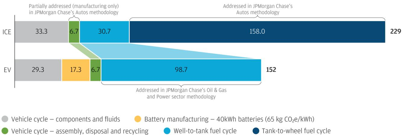
**Note:** Additional emissions with 80 kWh battery size consists of 2.6 t CO<sub>2</sub>e in vehicle cycle – batteries (65 kg CO<sub>2</sub>/kWh) and 1.4 t CO<sub>2</sub>-eq in 100 kg CO<sub>2</sub>/kWh battery manufacturing
